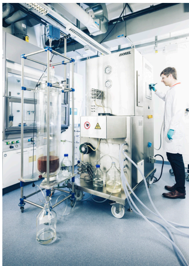
Lab-scale MES-RS in operation, © KIT, Karlsruhe
