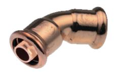
The fittings and tube shall be drawn from the Eco-Duo Copper Press fittings (available from Water Kinetics), manufactured from copper with EPDM 'O' rings. These fittings are for jointing copper tube and are available in sizes 15mm to 108mm. The fittings shall incorporate a "leak before press" facility offering a final check of the system to provide instant identification of joints that are assembled correctly but left unpressed. The fittings shall also offer electrical continuity.
