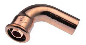
The fittings and tube shall be drawn from the Eco-Duo Copper Press fittings (available from Water Kinetics), manufactured from copper with EPDM 'O' rings. These fittings are for jointing copper tube and are available in sizes 15mm to 108mm. The fittings shall incorporate a "leak before press" facility offering a final check of the system to provide instant identification of joints that are assembled correctly but left unpressed. The fittings shall also offer electrical continuity.
