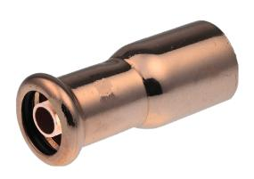
The fittings and tube shall be drawn from the Eco-Duo Copper Press fittings (available from Water Kinetics), manufactured from copper with EPDM 'O' rings. These fittings are for jointing copper tube and are available in sizes 28mm to 108mm. The fittings shall incorporate a "leak before press" facility offering a final check of the system to provide instant identification of joints that are assembled correctly but left unpressed. The fittings shall also offer electrical continuity.
