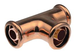
The fittings and tube shall be drawn from the Eco-Duo Copper Press fittings (available from Water Kinetics), manufactured from copper with EPDM 'O' rings. These fittings are for jointing copper tube and are available in sizes 15mm to 108mm. The fittings shall incorporate a "leak before press" facility offering a final check of the system to provide instant identification of joints that are assembled correctly but left unpressed. The fittings shall also offer electrical continuity.
