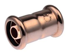
The fittings and tube shall be drawn from the Eco-Duo Copper Press fittings (available from Water Kinetics), manufactured from copper with EPDM 'O' rings. These fittings are for jointing copper tube and are available in sizes 15mm to 108mm. The fittings shall incorporate a "leak before press" facility offering a final check of the system to provide instant identification of joints that are assembled correctly but left unpressed. The fittings shall also offer electrical continuity.
