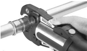
Fit jaw/sling jaws round EcoDuo fitting
