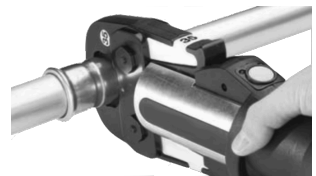
Press trigger/button Complete when closed
