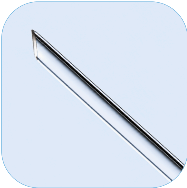
Actual Sunlight polar body biopsy pipette under microscopic magnification
