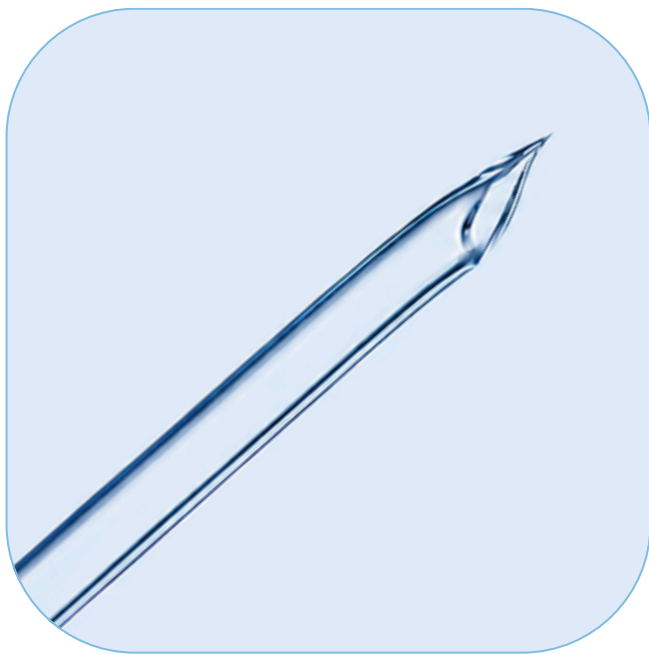
Actual Sunlight ICSI pipette under microscopic magnification
