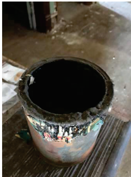
Photo 22: HA22 Roof tar (B62-B64). Access to the roof was unavailable, roofing materials were collected in the attic near the roof access ladder. 8% Chrysotile
