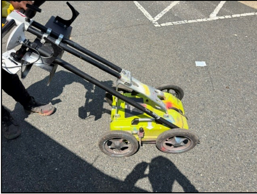
Photo showing the GPR cart utilized by the subcontracted GPR company.
