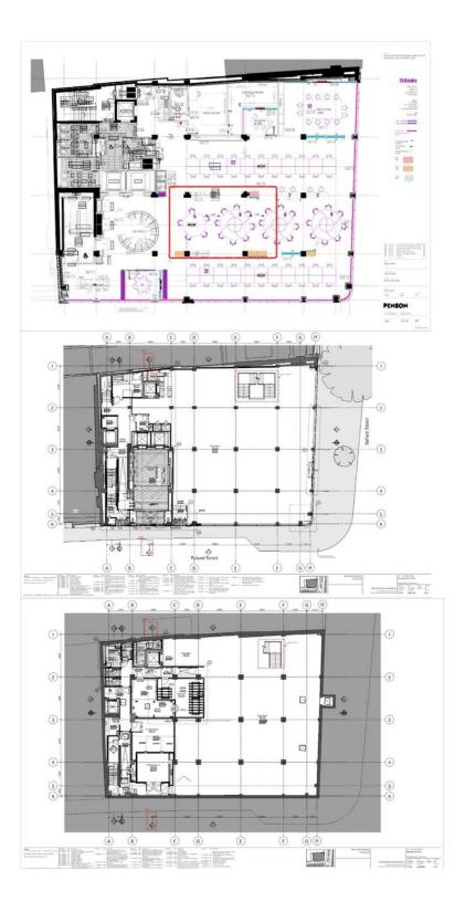
The above floor plans are for the surveying of 6th, 5th, 4th, 3rd & ground floor as well as basement. The one-way directional flow is clockwise vertically. Stair 1 is for descending and stair 2 is for ascending. The basement corridor is narrow and shared with retail staff for goods and people movement. Cooperation and coordination are required to minimise congestion.
