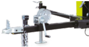
Manual cable winches for lift-up and tilt
