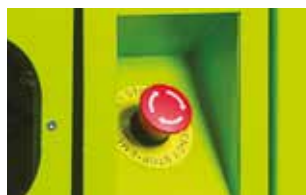
Niche for external emergency push-button
