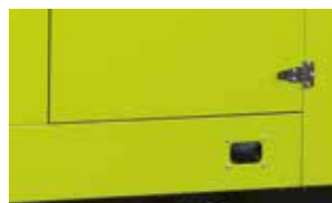
Opening for fuel pipes
