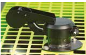
Exhaust silencer with rain flap
