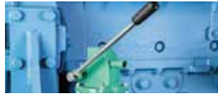
Manual lube oil drain pump
