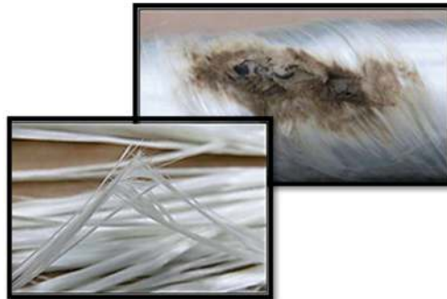
Figure A.6 – Breakage of Spiral-Wound Fibers Attributed to Cyclic Detrimental Impact Forces
