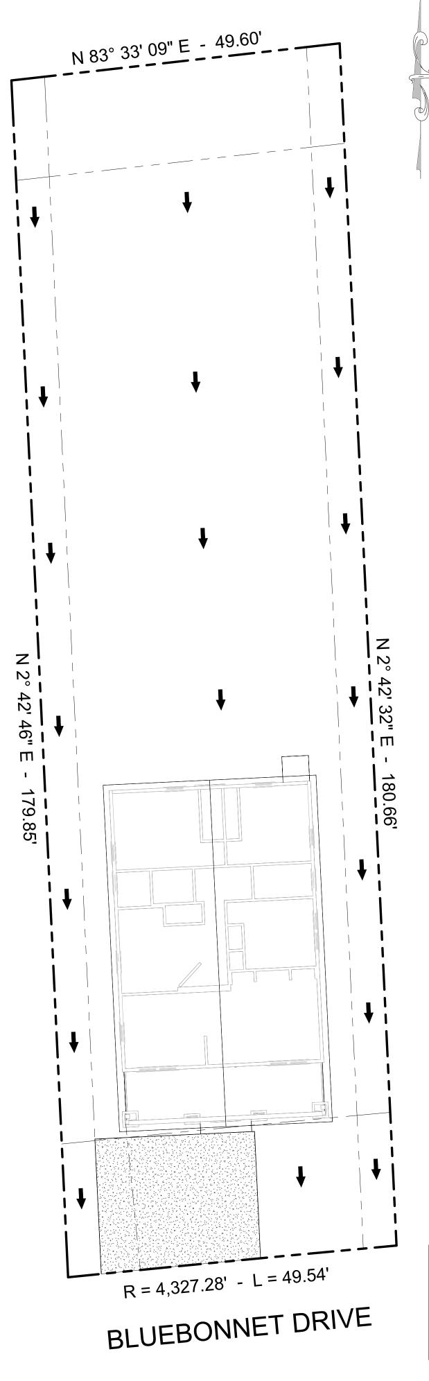
ENGINEER'S NOTE: NO FILL SHALL BE BROUGHT TO SITE. NO CHANGES SHALL BE MADE TO EXISTING GRADING OR DRAINAGE PLANS (AS-BUILT), AND THERE SHALL BE NO DRAINAGE IMPACT TO NEIGHBORHOOD PROPERTIES. CONTRACTOR/BUILDER SHALL BE 100% LIABLE FOR DEVIATION FROM THESE REQUIREMENTS BASED ON CITY INSPECTION.
