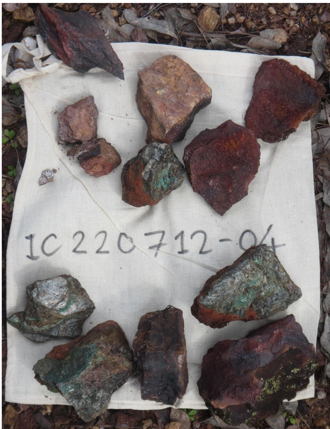
Sample IC220712-04, Effies Ace Area, 3.75% Cu, 1.05ppm Au, 4ppm Ag
