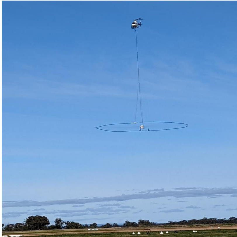
HeliTEM test flight, Tottenham aerodrome
