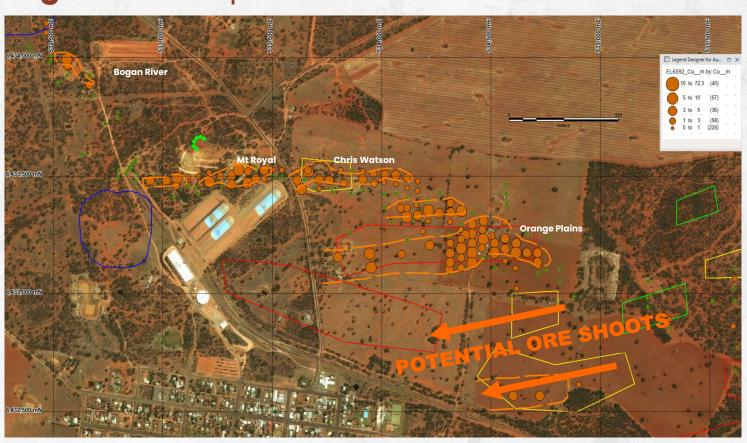
Tottenham area, %m Cu accumulation plot with 3%m Cu outline and modelled EM conductors
