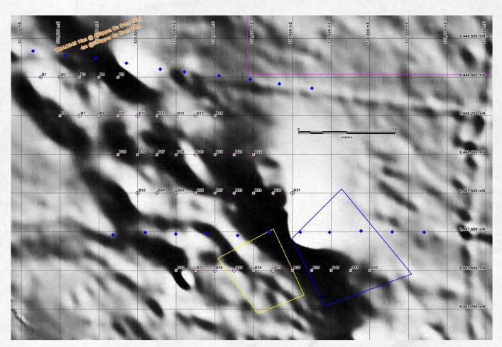
Reduced to pole magnetics, previous Mincor aircore drilling (blue crosses), airborne EM anomalies and proposed Locksley aircore. (MGA94 zone 55)
