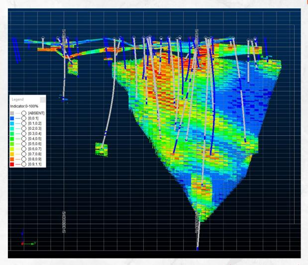
Visual validation of drill holes against model grade, long section looking west (Source: SnowdenOptiro)
