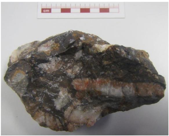
Sample IC220826-11; Iron oxide matrix fault breccia, Lacey's Tank Prospect (MGA 94 zone 55 532614mE 6439259mN), 0.38ppm Au, 0.18% Cu
