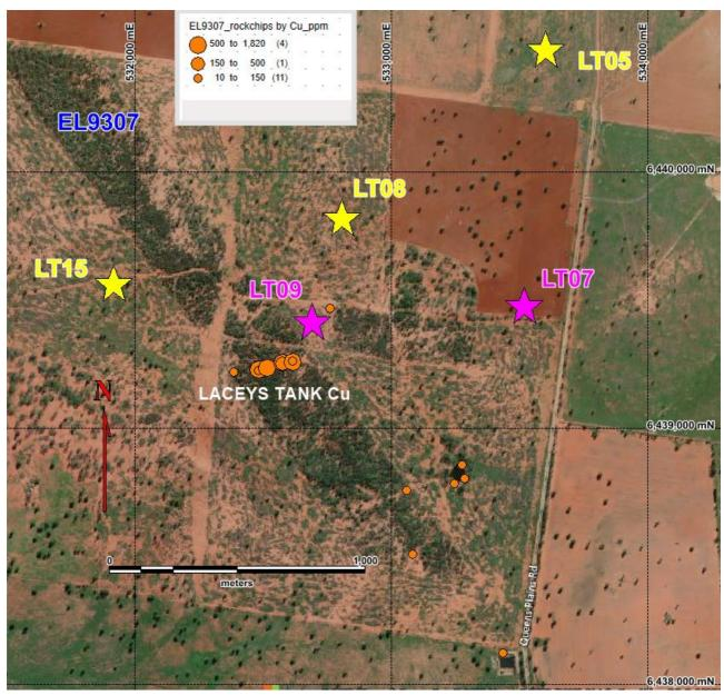
Laceys Tank HeliTEM anomalies and rock chip samples. (Map Grid Australia zone 55)
