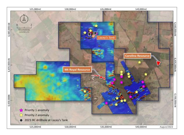
Figure 11. Tottenham Project – Historic drillholes and ranked HeliTEM<sup>2</sup> anomalies in the Tottenham area with current resources shown in orange
