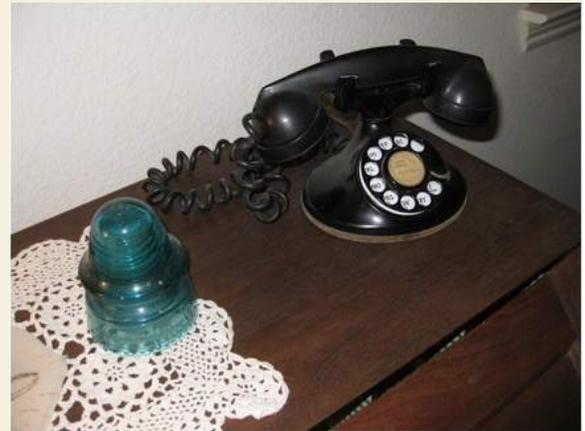
This is the telephone that served our family during the *Hungry Hollow Telephone Company* existence. The green insulator is one used to hold the wires up on the pole. Circa 1940's.
