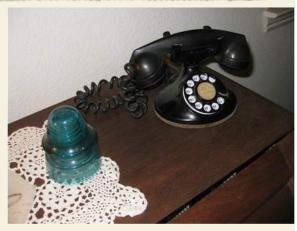
This is the telephone that served our family during the *Hungry Hollow Telephone Company* existence. The green insulator is one used to hold the wires up on the pole. Circa 1940's. Bill Rominger
