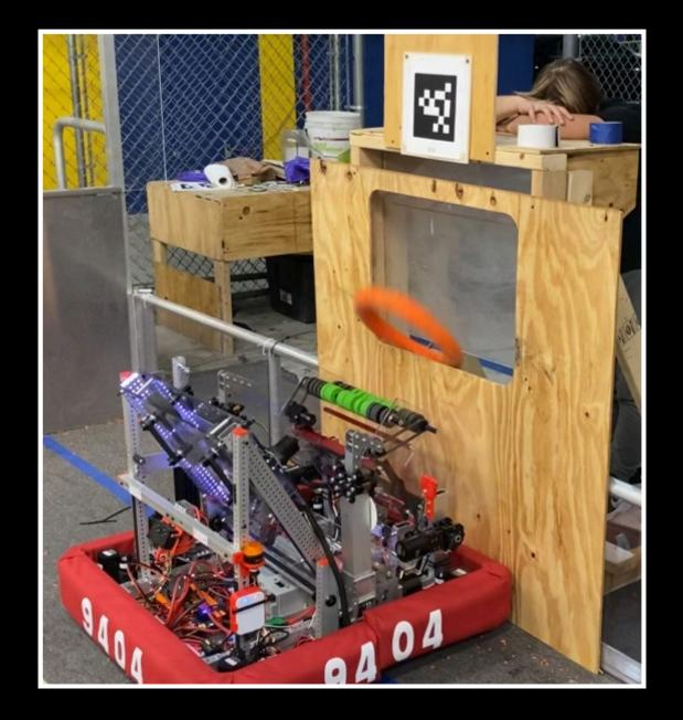
Automated Amp Scoring based off on our predetermined Encoder value to find the best position and speed to score into the Amp.
