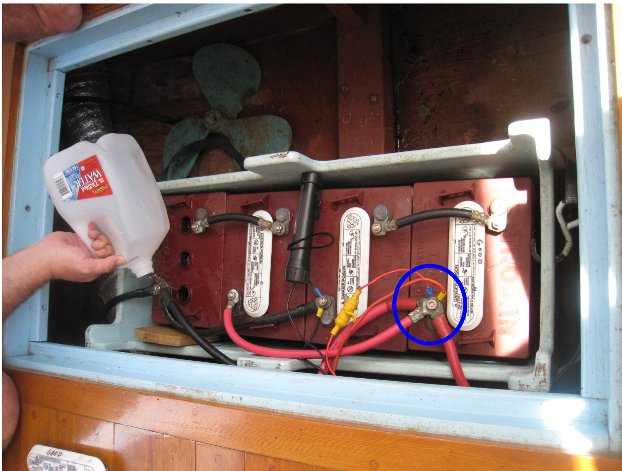
House battery bank being topped off with water. Per ABYC E-11. No more than four (4) terminals shall be mounted to a single battery stud.
