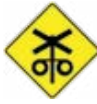
Railway level crossing – flashing signal ahead
