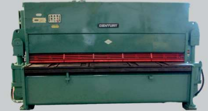
Sheet shearing Cincinnati max cal 3/8 x 10' of sheet metal.
