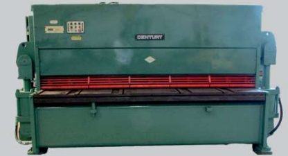
Sheet shearing Cincinati max cal 3/8 x 10' of sheet metal.
