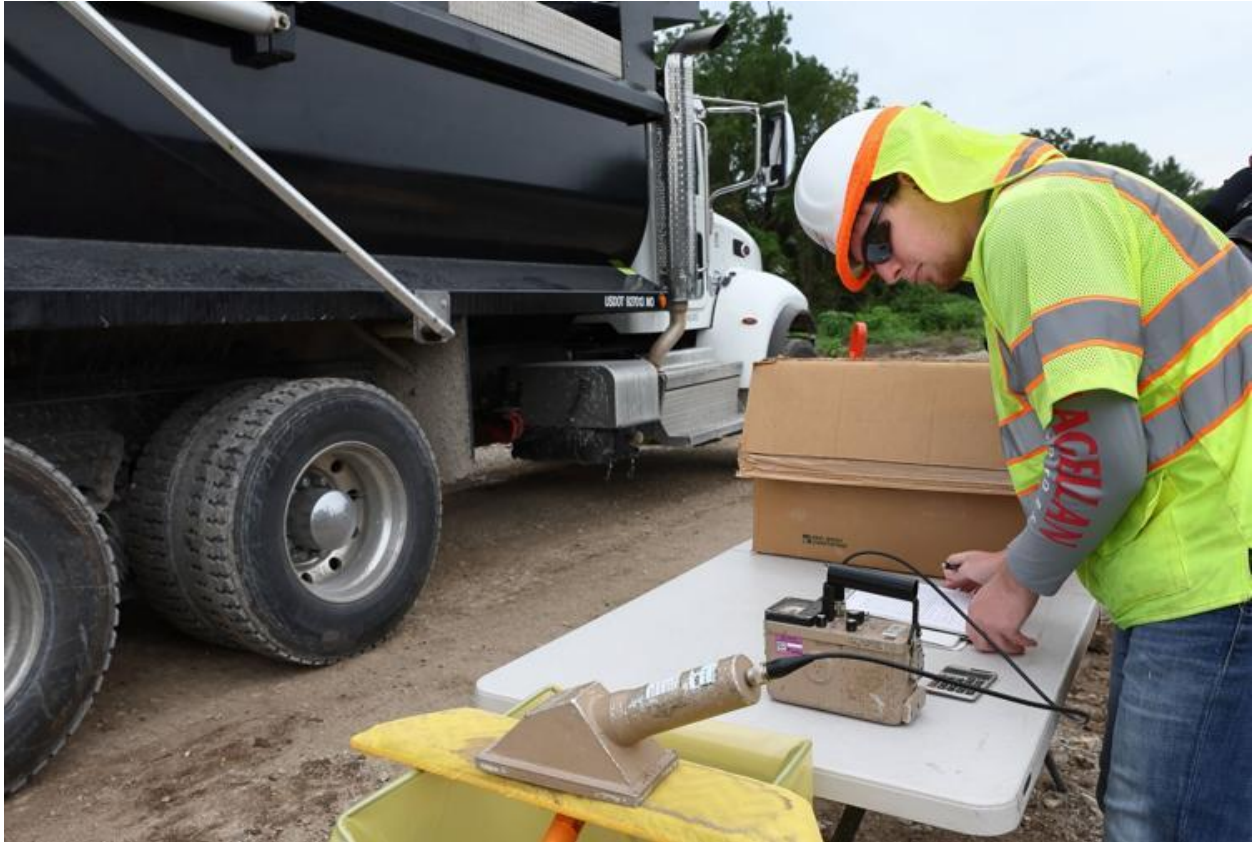
Caleb Hansen, a radiation protection tech, tests a cloth he used to wipe down a dump truck carrying away soil contaminated with radioactive waste from the banks of Coldwater Creek near Jana Elementary School in Florissant on Tuesday, Sept. 5, 2023. David Carson, Post-Dispatch
