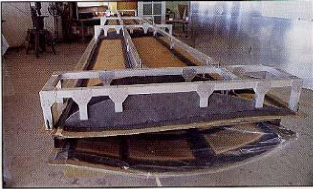
Rib alignment jig.
