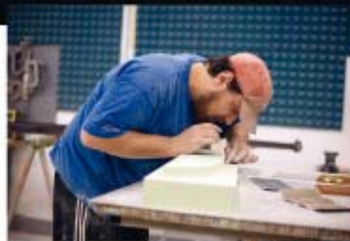
Last preparations before the wing finds its way into the oven. Foil and fabric protect the actual component.
