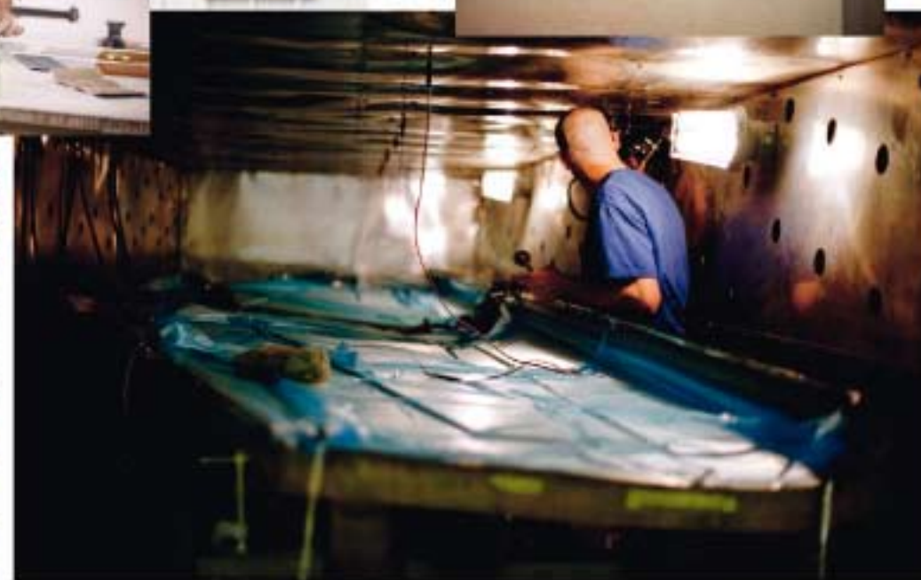
The V3’s strongest part (left). This part of the wing can withstand 34G. Baking time (above). The wing sizzles for almost four hours, first at 70 °C, then once the parts are joined, the heat goes up to 120°.
