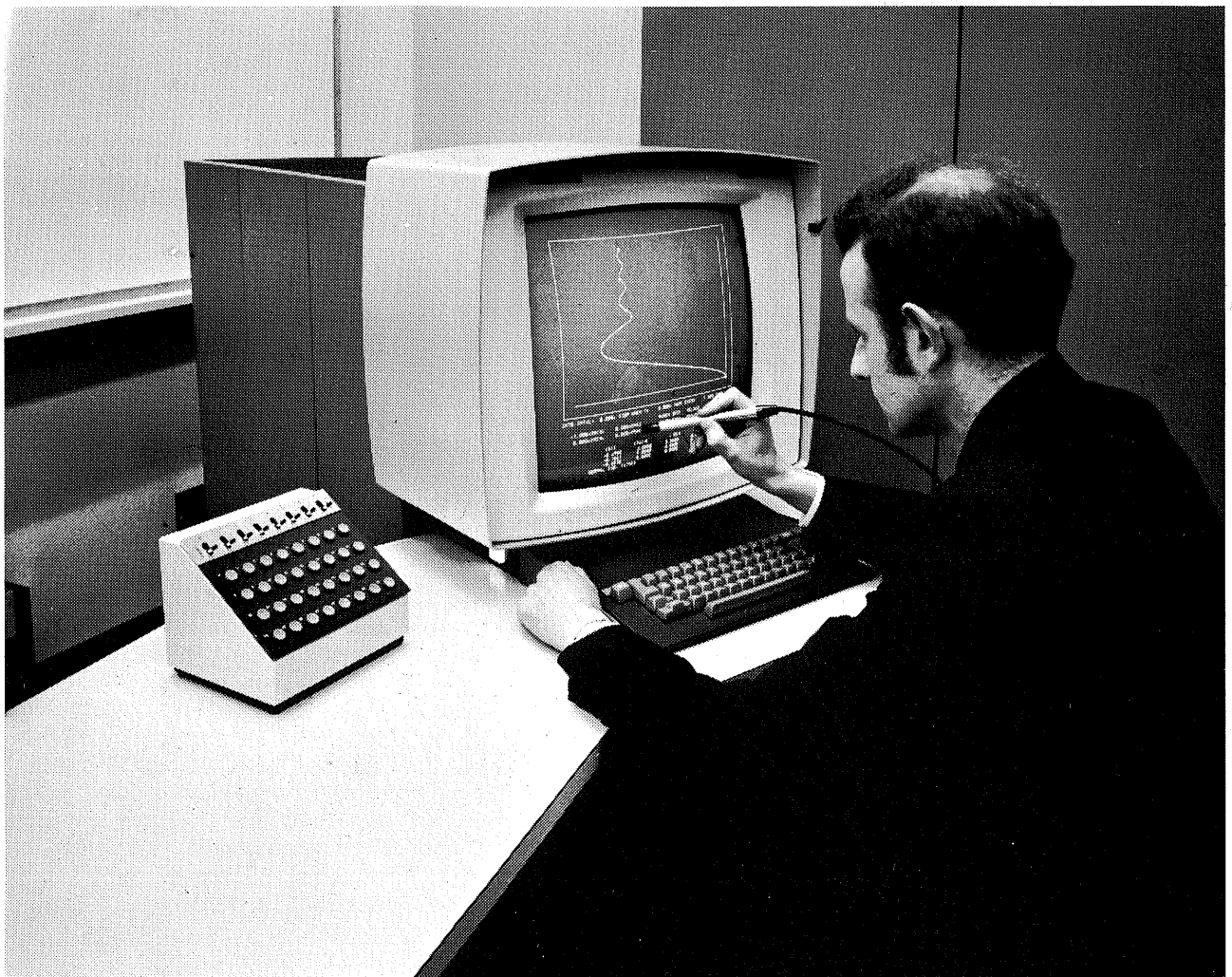
Plate 2. A typical line drawing unit. The operator is using the light pen held in his right hand to actuate a 'menu' of light buttons displayed on the screen. He may also use the keyboard below the screen and the function diagrams may be produced on a graph plotter (see plate 1).
