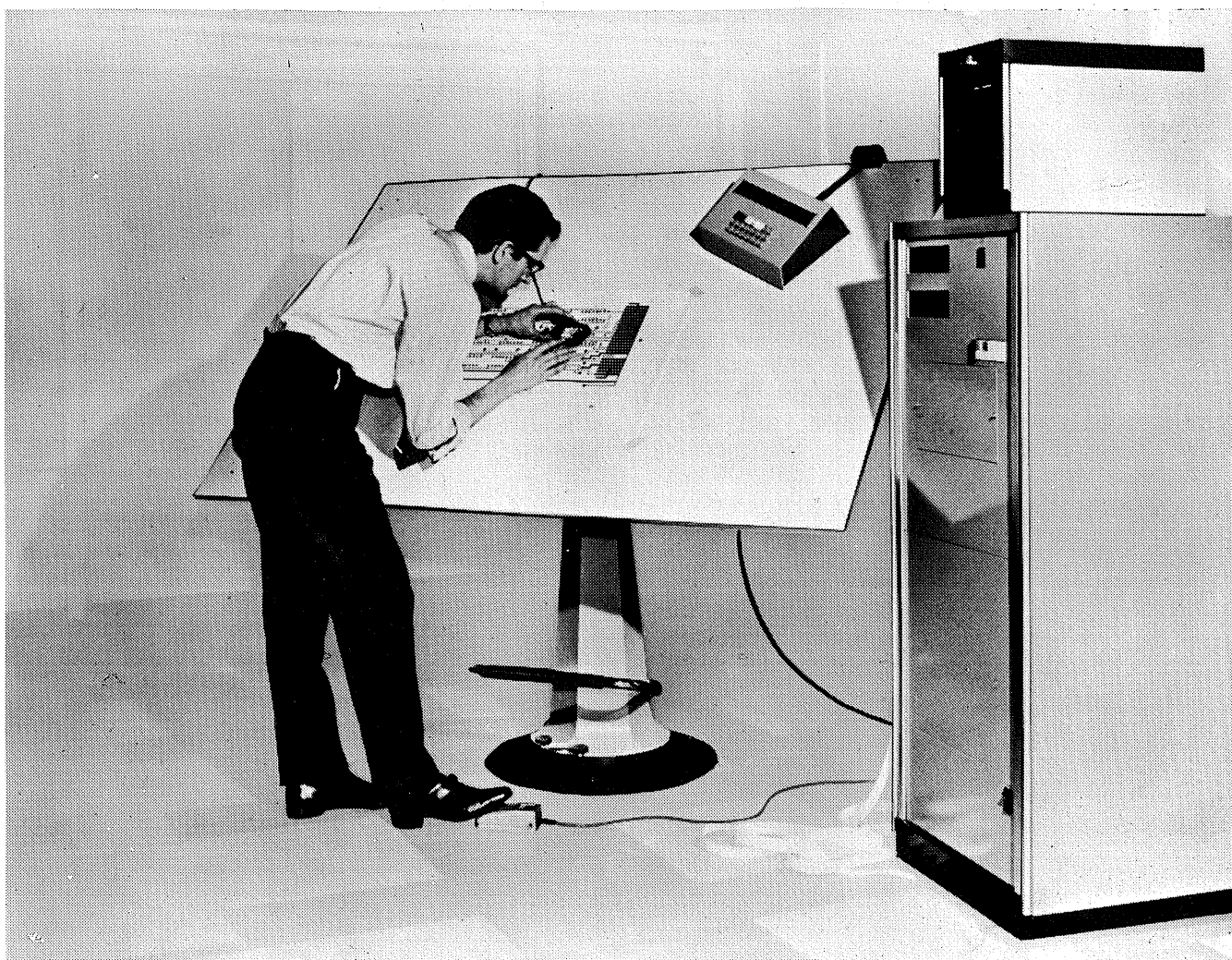
Plate 3. A digitising table. The operator is using the 'pencil' (lens and cross wires) and footswitch to produce coordinate pairs for input to the computer. The keyboard (top right of table) is used for punching alphanumeric titles for identification purposes.
