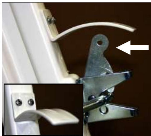
Step 2: Position latch shield above gate latch & check that latch has room to operate properly. Center shield & secure with 2 - #10 x 3/4 screws provided
