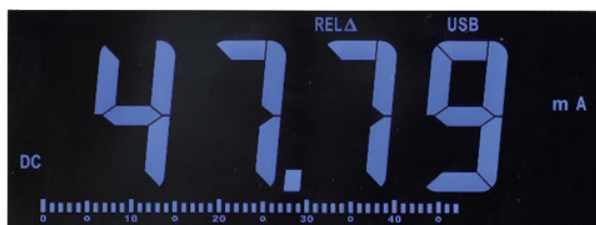
Extreme value operation and reference value operation function, with analog bar
