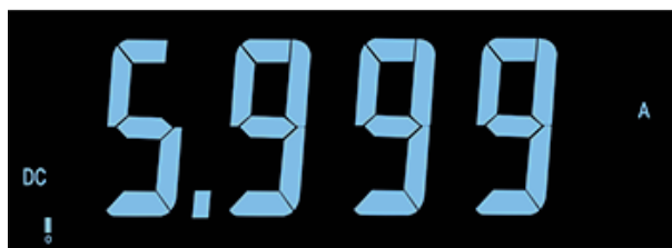
Reading resolution 3½ digits. Maximum count 5,999
