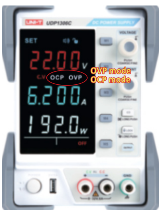
Over voltage/current/temperature protection
