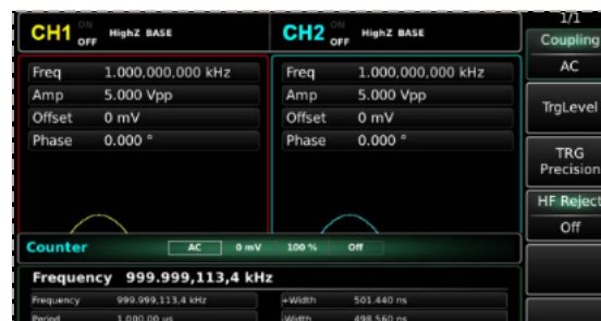
Frequency counter from 100mHz to 200MHz
