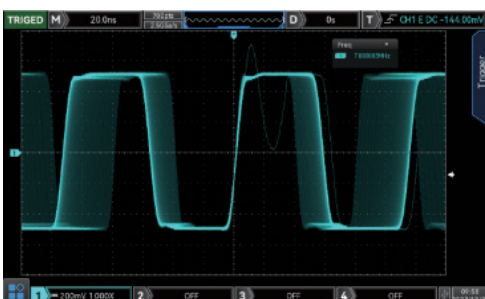
Ultra high capture rate 1,000,000 wfms/s in Fast Acquire mode
