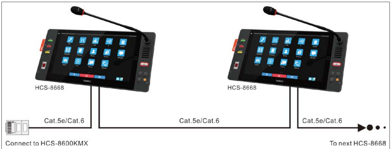
Figure 3.2.7 Daisy-chain connection between HCS-8668/8638 series Paperless Multimedia Congress Terminals
