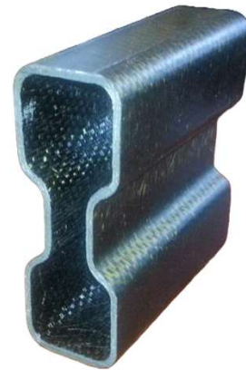
Example PMC net lay-up closed shape forming
