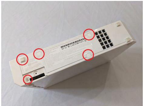
6) Flip the Wii so the bottom is facing upwards. Remove the two rear rubber feet and the two adhesive screw covers in the front. Unscrew the phillips screws in the front and the tri-wing screws in the back.
