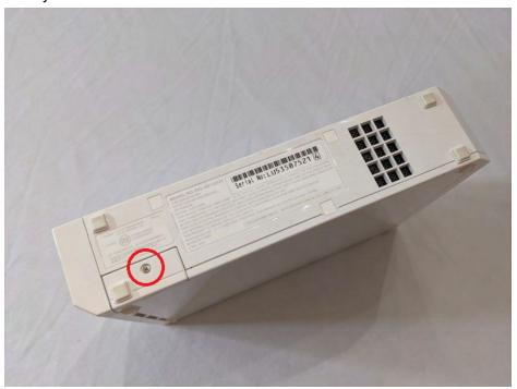
5) Remove the front rubber foot, and the three adhesive screw covers. Use a hobby knife to get under the screw covers. Unscrew the phillips and tri-wing screws.
