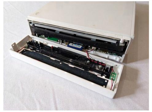
8) Remove the top cover of the Wii by pulling upwards on it.
