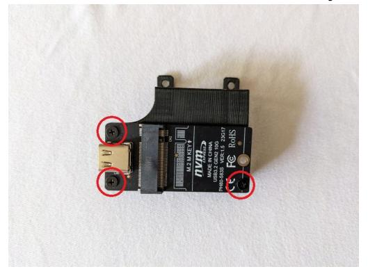
10) Install the 2230 NMVe drive onto the PCB. Install the drive spacer/nut and screw. The chamfered inner hole goes upward (which seems backwards). Insert the USB C cable into the PCB as well.
