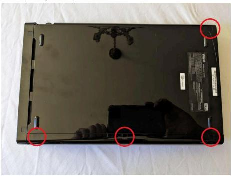
2) Remove the three screws along the side.
