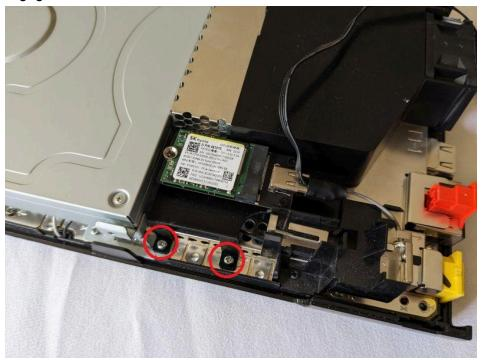
12) Route the USB cable over to the other side of the Wii U and plug in the USB A side.
