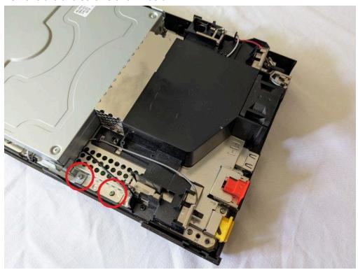
9) Grab the SSD PCB mount and PCB board. Screw in the three mounting screws.
