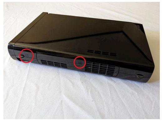
7) Pull up on the back of the Wii U top cover, then slide it back to remove it.
