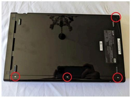
5) Unscrew and remove the battery from the side of the Wii U.
