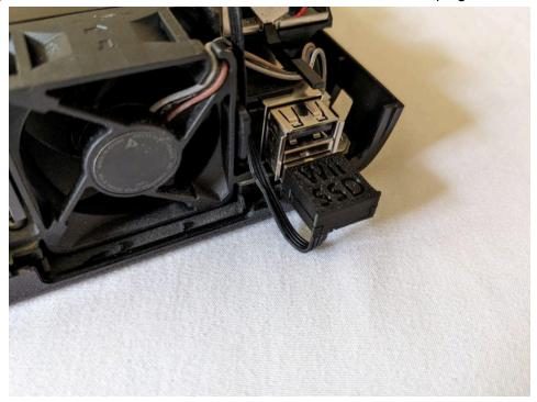
13) Grab the Wii U top cover. Remove the fan grill from the back by sliding it out.. Replace it with the included fan grill. Orient it so that the small cutout is in the lower right corner.
