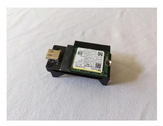
11) Install the NVMe2WiiU into the rear corner of the Wii. Reinstall the two screws that you previously removed. Do not tighten them down very tight as there is now less thread engagement.
