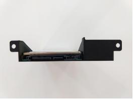
3) Slide the sled / spacer and hard drive into the Playstation 2 hard drive bay.
