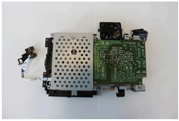
14) Remove the 4 phillips screws holding the power board to the chassis.
