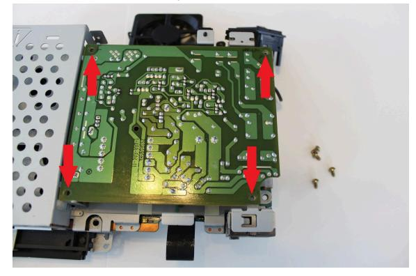
15) Pull the power board straight up to release it from the main board. Place it to the side.
