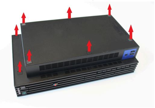
4) Use the phillips screwdriver to remove the 8 screws from the case.
