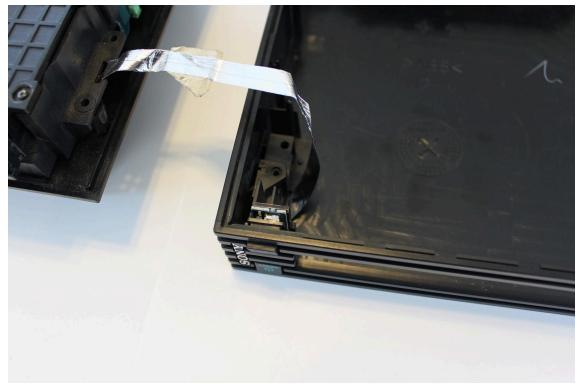
28) Reinstall the top cover. Slide the front cover over the controller ports and cd tray, then angle it down in the reverse order as disassembly.
