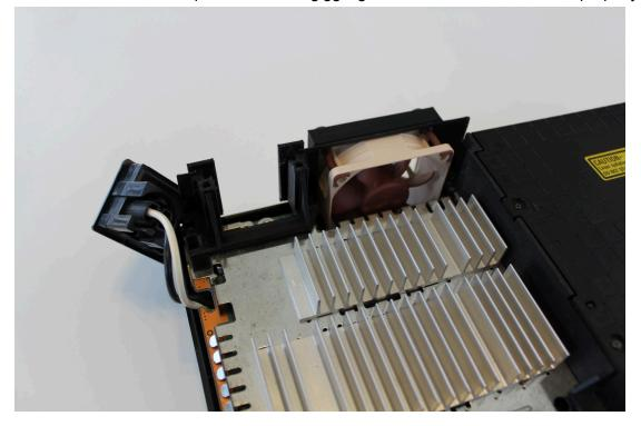
24) Slide the power switch assembly down into the back plate. Reinstall the back plate screw.
