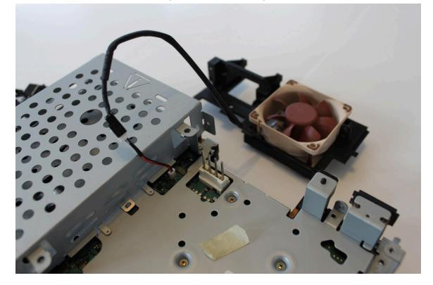
19) Reuse the tape to hold down the new fan wires. If the tape was torn in disassembly you can use new tape. How the fan wire is routed is not important as long as it does not interfere with reassembly.
