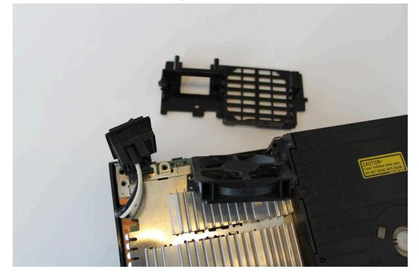
11) On the back side of the console, remove the expansion bay panel.
