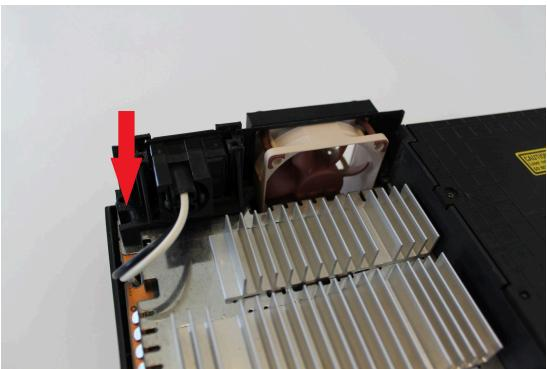
25) Reconnect the ribbon cable to the controller board.
