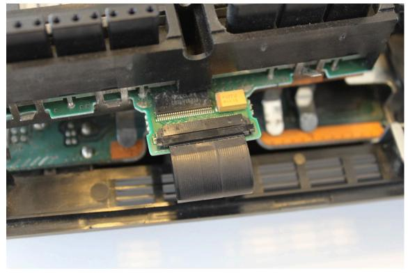
26) Reinstall the controller board and reinstall the two screws.
