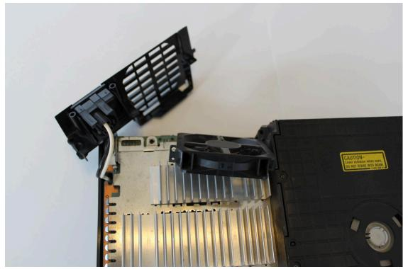
9) Pull the case fan up and out of the back plate. Then pull up and remove the back plate.
