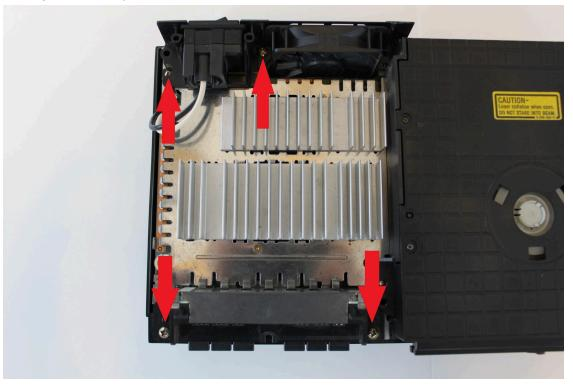
8) Pull the controller board up gently. There is a ribbon cable attached to it. Gently pull / flip / rotate up the connector to release the ribbon cable. Place the board to the side.
