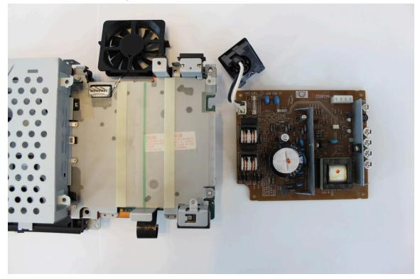
16) Remove the plastic insulation sheet and place it to the side.
