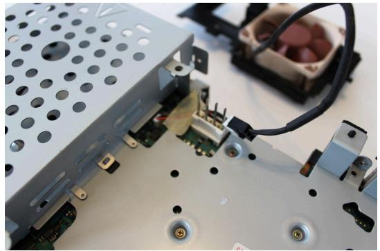
20) Replace the plastic insulation sheet.
