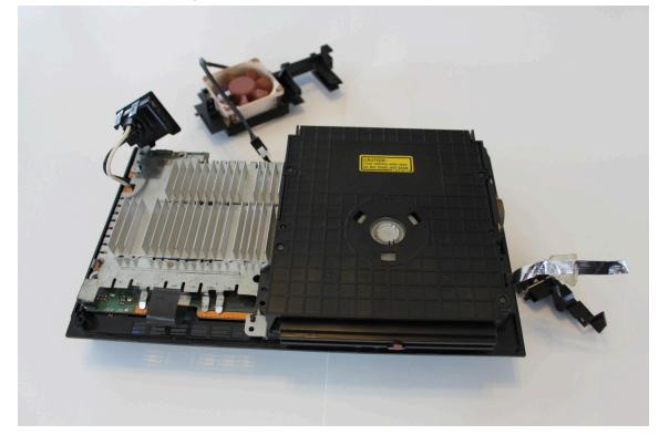
23) Install the fan modification back plate. The fan wire should be pushed in the case as needed. Some cases require a fair bit of giggling the mod around for it to seat properly.
