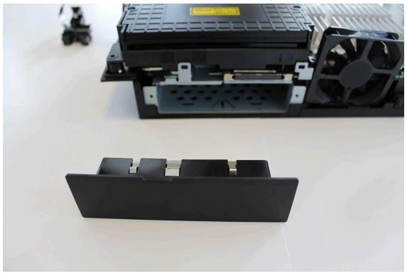
12) Lift the inner assembly out of the lower case.
