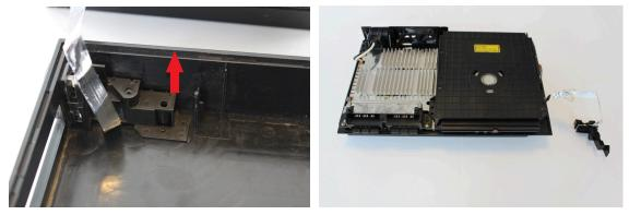
7) Remove the two phillips screws that hold the back panel and fan in, and the two screws holding the memory card and controller board.
