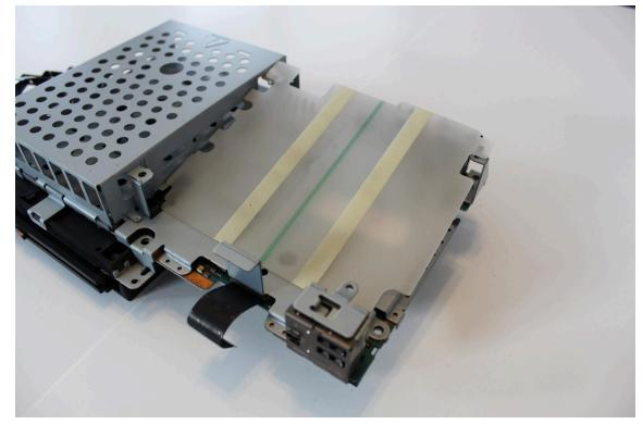
17) Remove the fan wire tape. Unplug the fan and set it to the side.
