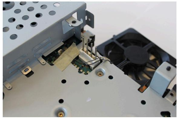
18) Take the fan modification and plug the fan into the plug on the console board.
