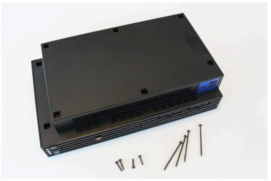
5) Pull up on the console case from the back side tilting it toward the front. Once it is loose, flip the left side up and to the right.
