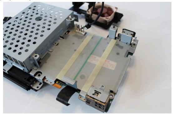
21) Push the power board straight down onto the main board making sure to line up the 4 pin connector. Replace the 4 screws that hold it to the chassis.
