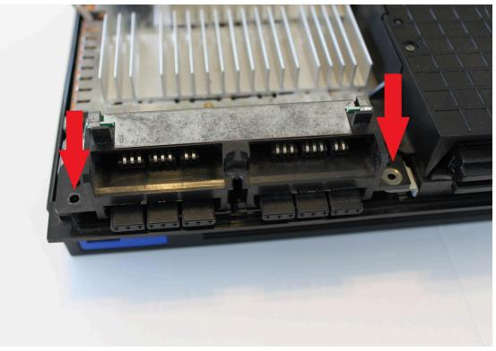
27) Reinstall the power switch into the upper cover. Slide it into place and push down.
