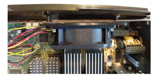
12) Push down on the fan assembly to lock it in place. Make sure the fan does not get hung up on the main board. The fit is on the tighter side.
