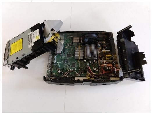
8) Unplug the original fan power connector by pulling up on it.
