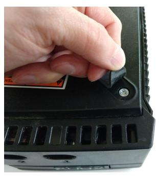
3) Turn the console rightside up again. Grab the top half and pull up on it to slide it off of the bottom.
