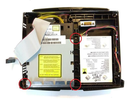
6) Pull up on the hard drive platform and flip it over the side of the Xbox.
