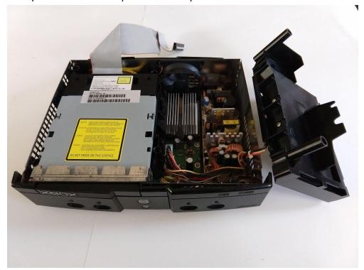
7) Pull up on the optical drive platform and move it over the side of the Xbox.
