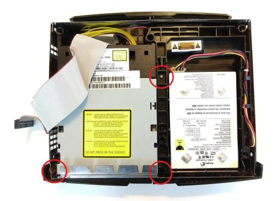
18) Plug the grey IDE cable back into the hard drive. Tuck it into the retaining clip.
