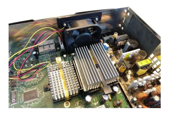
13) Grab the CPU block and place it on the CPU heatsink. This redirects more air over the GPU which runs hotter than the CPU. Oddly enough, this does not actually make the CPU run hotter.
