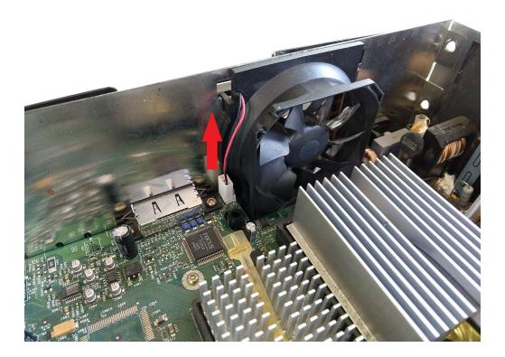
9) Locate the tabs on either side of the original fan. Pry one or both of these with a screwdriver while pulling up on the fan. Some force may be needed to release the fan. After the fan pops up a little bit, pull it away from the back of the case to pull the fan tabs through the back plate. This will fully remove the fan.
