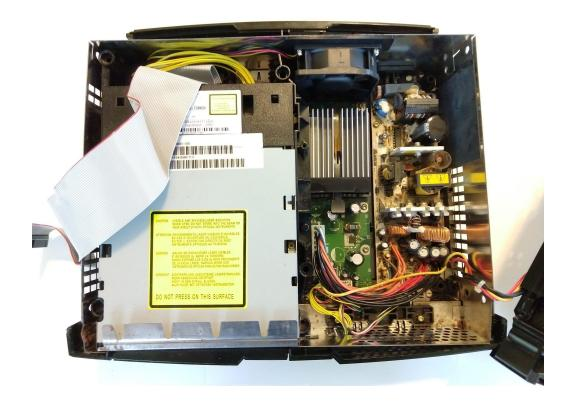
15) Tuck the fan wires back behind the yellow wires for a tidier installation.
