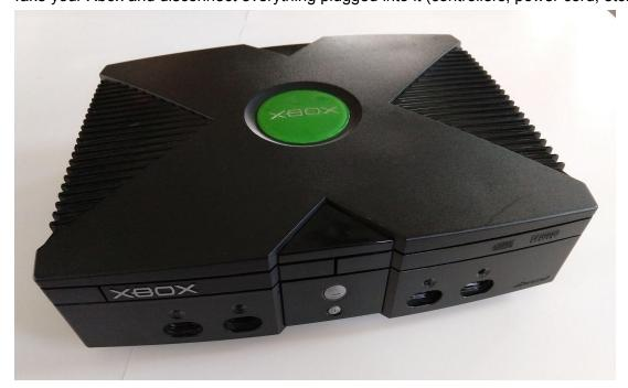
2) Turn the console upside down. There are six T20 torx screws to remove. The center two are under stickers. The four on the corners are under the outer side of the rubber feet.
