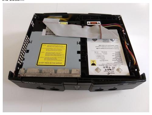
4) Remove the grey IDE cable from the back of the hard drive. It pulls straight out of the back of the hard drive. There are no clips.
