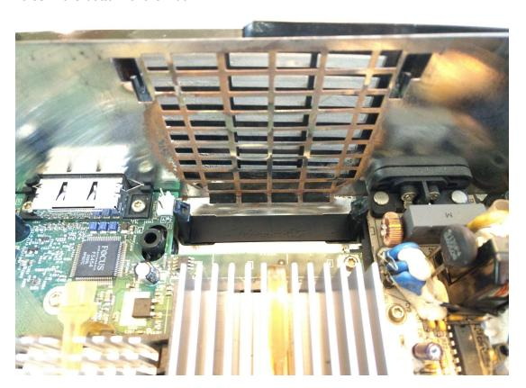
11) Grab the new fan and mounting plate assembly. Plug the fan power connector into the Xbox main board. Then, place the tabs on the mounting plate through the back plate of the Xbox.
