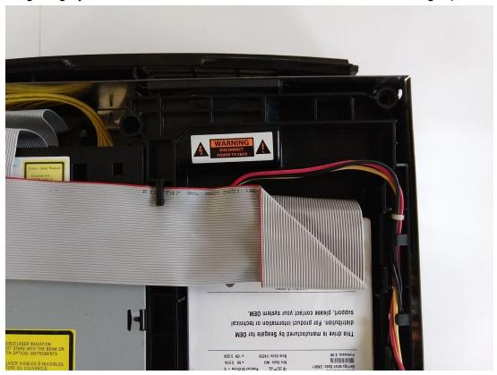
19) Slide the top cover down on top of the lower half of the Xbox.
