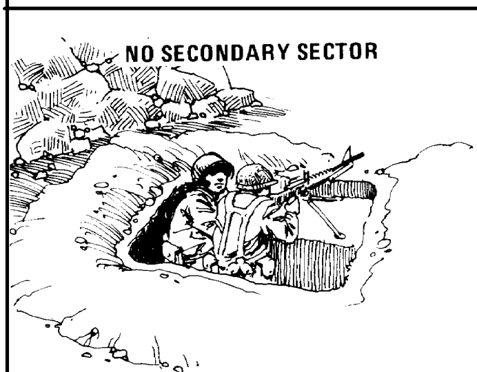
IN SOME POSITIONS, AN MG MAY NOT HAVE A SECONDARY SECTOR OF FIRE; SO, ONLY HALF OF THE POSITION IS DUG.
