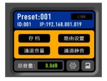
After connecting the device with a network cable, the computer's IP address needs to be in the same network segment as the device's IP. If it is not in the same network segment, the IP address needs to be modified (for example, modify it to 192.168.1.33)
