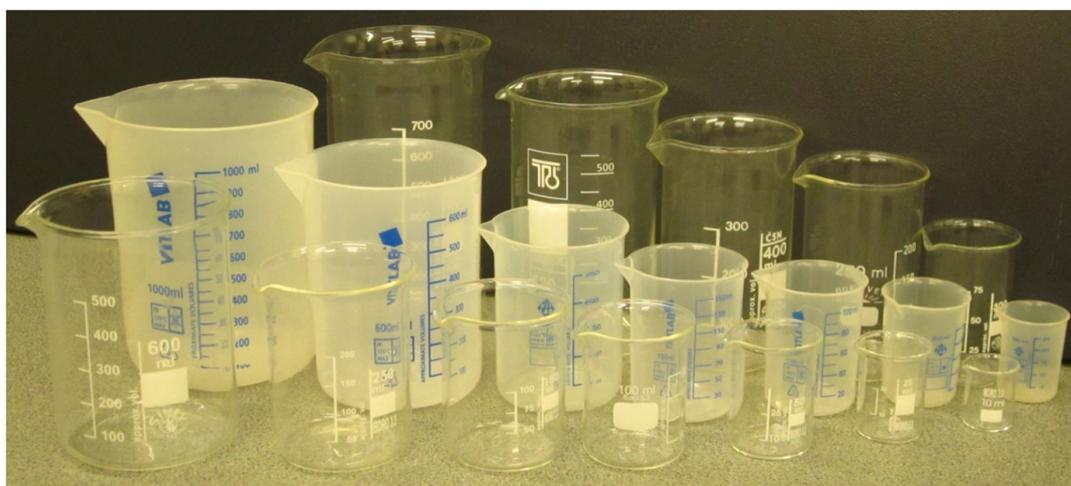
Figure 1.4. Glass and plastic beakers of different size.
