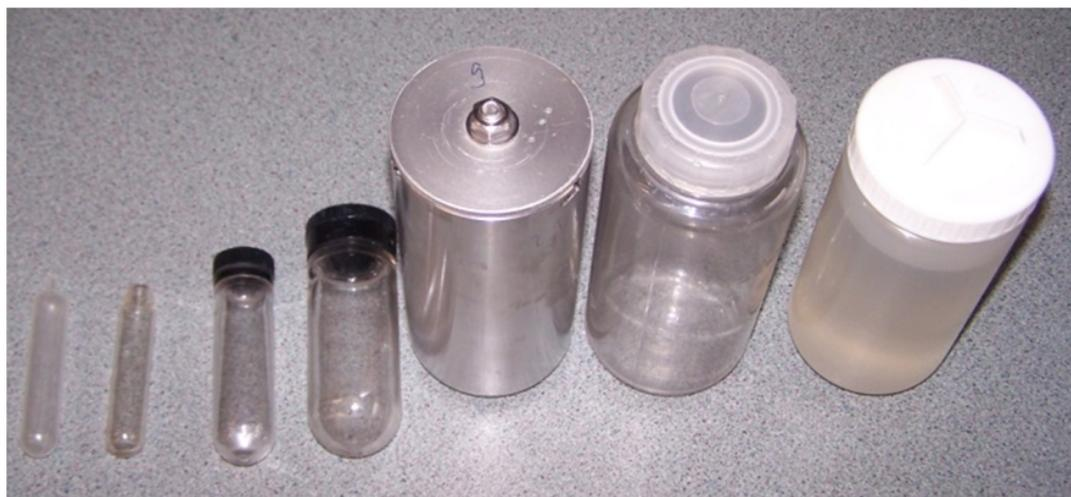
Figure 1.16. Centrifuge tubes.
