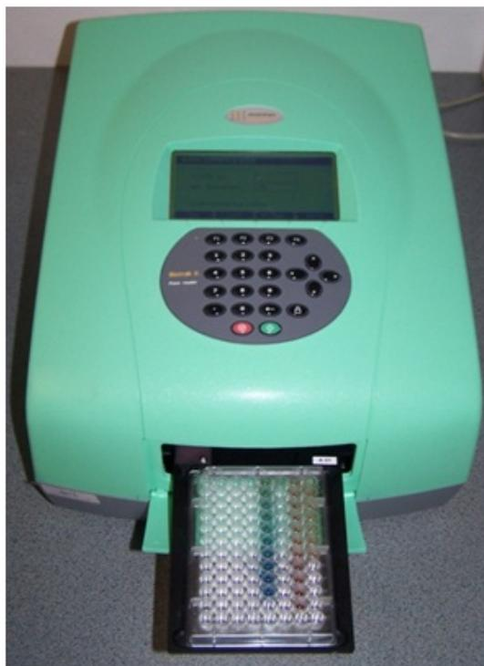
Figure 4.4. Plate reader with a 96-well plate
