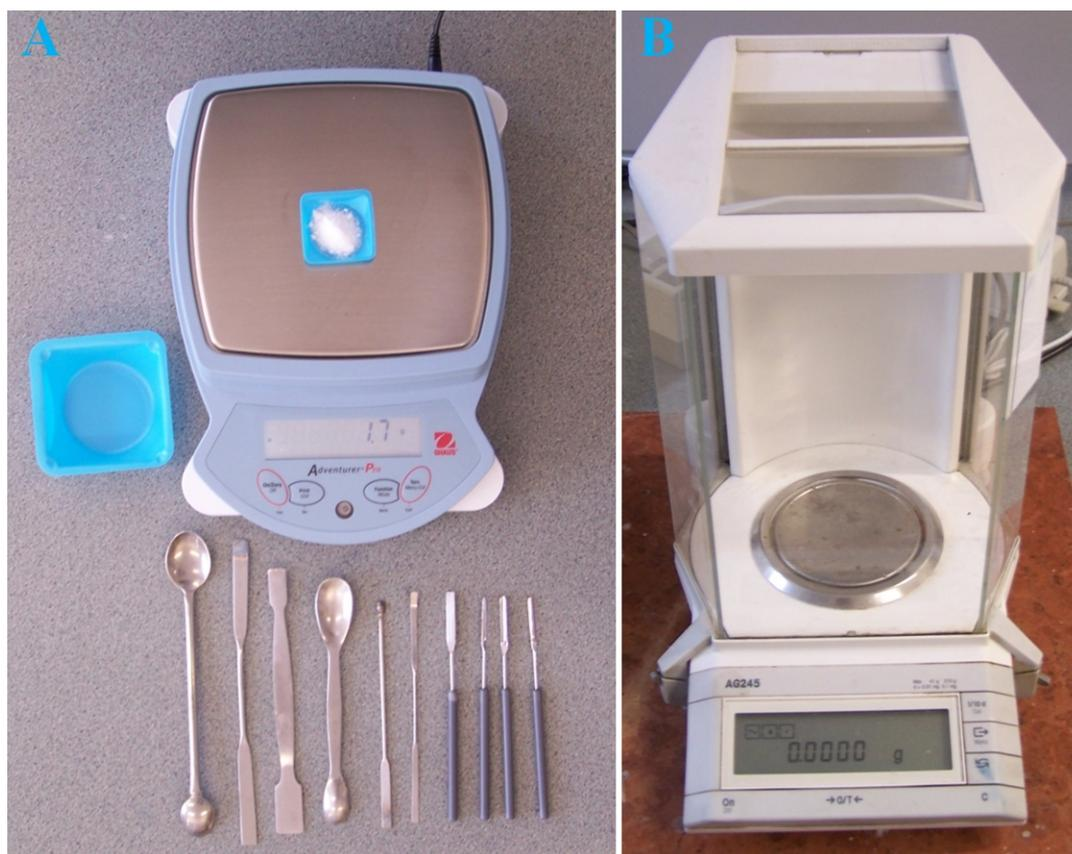
Figure 1.11. A, Top loading balance with disposable weighing dishes, laboratory spatulas and spoons. B, Analytical balance on a vibration-free surface.
