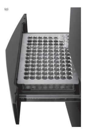
Fig. 14.4 (a) Geiger–Müller bench monitor; (b) liquid scintillation counter; (c) sample rack for liquid scintillation counter. (Reproduced with permission from LabLogic; instrument shown is the Hidex 300SI.)
