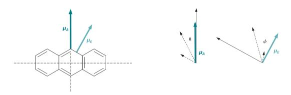
Fig. 12.15 Absorption dipole moment  $\mu_A$  (describing the probability of photon absorption) and transition dipole moment  $\mu_E$  (describing the probability for photon emission) for any chromophore are usually not parallel. Absorption of linearly polarised light varies with  $\cos^2\theta$  and is at its maximum parallel to  $\mu_A$ . Emission of linearly polarised light varies with  $\sin^2\phi$  and is highest at a perpendicular orientation to  $\mu_E$ .
