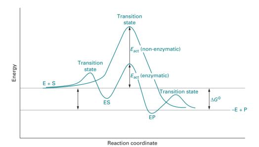
Fig. 15.7 Energy profile of a simple enzyme-catalysed reaction. The formation of ES and EP and the subsequent release of E+P proceeds via several transition states. The activation energy for the overall reaction is dictated by the initial free energy of E and S and the highest energy transition state. The non-enzyme-catalysed reaction proceeds via a higher energy transition state and hence the reaction has a higher activation energy than the enzyme-catalysed reaction.
