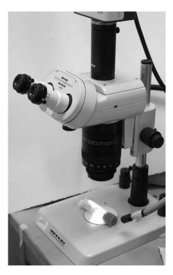
Fig. 4.6 A research-grade stereomicroscope. Note the light source is from the side, which can give a shadow effect to the specimen; in this example a vial of fruit flies. The large objective lens above the specimen can be rotated to zoom the image.
