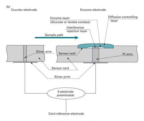
Fig. 16.2 Micro sensor analyte detectors. (a) The GEM 3000 Sensor Card; (b) the Amperometric Glucose/Lactate Analyte Sensors. (Reproduced by permission of IL Critical Care, Lexington, USA.)
