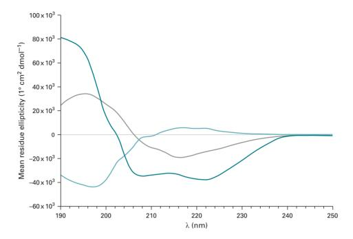
Fig. 12.18 Circular dichroism spectra for three standard secondary structures according to Fasman. An  $\alpha$ -helical peptide is shown in dark green, a peptide adopting β-strand structure in grey, and a random coil peptide in light green.
