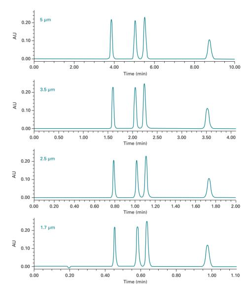
Fig 11.7 Chromatograms showing the influence of particle size on the resolution and elution time of four analytes in an HPLC system demonstrating the time advantages of the pressure-tolerant sub-2  $\mu$ m ACQUITY UPLC system. (Reproduced by permission of Waters Corporation, UK.)
