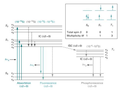
Fig. 12.8 Jablonski diagram. Shown are the electronic ground state ( $S_0$ ), two excited singlet states ( $S_1$ ,  $S_2$ ) and a triplet state  $(T_1)$ . Vibrational levels (v) are only illustrated exemplarily. Solid vertical lines indicate radiative transitions, dotted lines show non-radiative transitions. The inset shows the relationship between electron configurations, total spin number S and multiplicity M.
