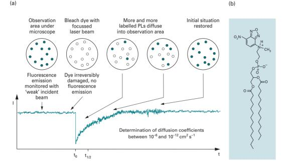
Fig. 12.13 (a) Schematic of a FRAP experiment. Time-based monitoring of fluorescence emission intensity enables determination of diffusion coefficients in membranes. (b) A commonly used fluorescence label in membrane FRAP experiments: chemical structure of phosphatidylethanolamine conjugated to the fluorophore NBD.
