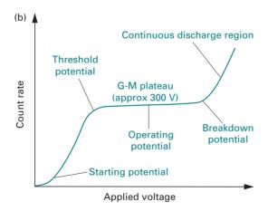
Fig. 14.3 (a) The Geiger-Müller (G-M) tube and (b) the effect of applied voltage on count rate.
