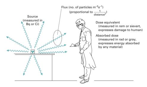
Fig. 14.11 The relationship between radioactivity of source and absorbed dose.
