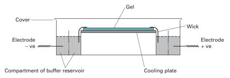
Fig. 10.2 A typical horizontal apparatus, such as that used for immunoelectrophoresis, isoelectric focussing and the electrophoresis of DNA and RNA in agarose gels.
