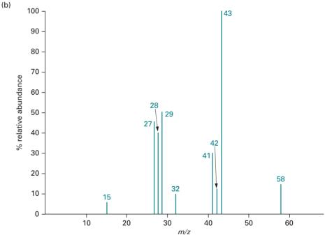
Fig. 9.3 Fragmentation pathways in *n*-butane and the EI spectrum. The pathway for fragmentation of *n*-butane is shown in (a) and the EI spectrum in (b). In the spectrum, the relative abundance is plotted from 0 to 100% where the largest peak is set at 100% (base peak). Spectra represented in this way are said to be **normalised**.
