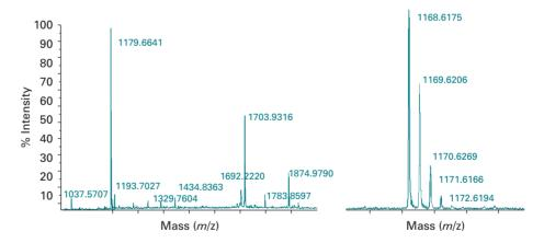
Fig. 9.13 Two examples of MALDI–TOF peptide spectra. The left-hand spectrum is from a protein digest mixture and the right-hand image is an expanded one of a small part of a spectrum showing <sup>13</sup>C-containing forms (see Section 9.5.4).
