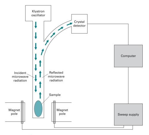
Fig. 13.5 Diagram of an EPR spectrometer.
