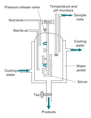
Fig. 2.13 Schematic representation of a fermenter.
