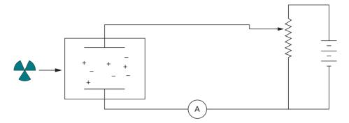
Fig. 14.2 Detection based on ionisation.
