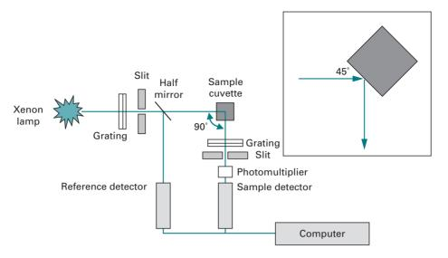
Fig. 12.9 Schematics of a spectrofluorimeter with 'T' geometry (90°). Optical paths are shown as green lines. Inset: Geometry of front-face illumination.
