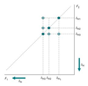
Fig. 13.10 Schematics of a correlated 2D-1H NMR spectrum. H3 couples with H2 and H1. H1 and H2 show no coupling.
