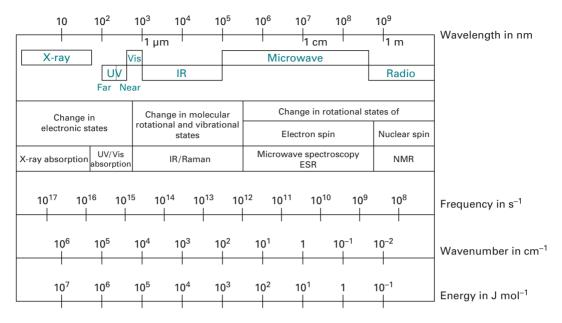
Fig. 12.2 The electromagnetic spectrum and its usage for spectroscopic methods.
