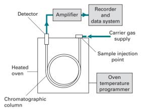
Fig. 11.12 Components of a GC system.
