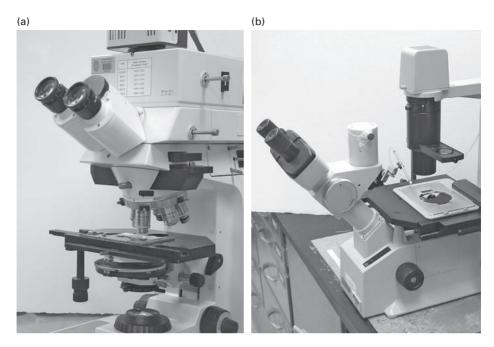
Fig. 4.3 Two basic types of compound light microscope. An upright light microscope (a) and an inverted light microscope (b). Note how there is more room available on the stage of the inverted microscope (b). This instrument is set up for microinjection with a needle holder to the left of the stage.
