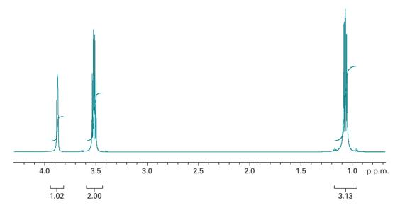
Fig. 13.8 <sup>1</sup>H NMR spectrum of ethyl alcohol (H<sub>3</sub>C–CH<sub>2</sub>–OH) with integrated peaks.
