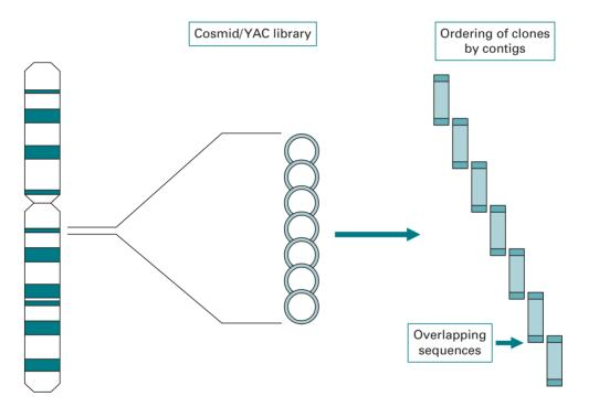
Fig. 6.47 Physical mapping using continuous overlapping cloned fragments (contigs). In order to assign the position of cloned DNA fragments resulting from the construction of a library in a YAC or cosmid vector, overlaps are detected between the clone fragments. These are created because of the use of partial digestion conditions when the libraries are constructed.
