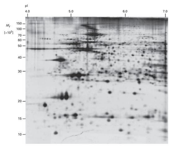
Fig. 10.9 A typical two-dimensional gel. The sample applied was 100 μg of total protein extracted from a normal dog heart ventricle. The first dimension was carried out using a pH 4–7 isoelectric focussing gel. The second dimension was a 12% SDS–PAGE vertical slab gel. The pattern was visualised by silver staining. (Courtesy of Monique Heinke and Dr Mike Dunn, Division of Cardiothoracic Surgery, Imperial College School of Medicine, Heart Science Centre, Harefield, UK.)
