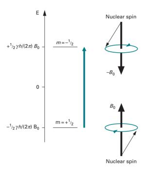
Fig. 13.7 Energy levels of a proton in the magnetic field  $B_0$ . The nuclear spin of a nucleus is characterised by its magnetic quantum number m. For protons, m can only adopt  $+\frac{1}{2}$  and  $-\frac{1}{2}$ . The corresponding energies are calculated by  $-m\gamma hI(2\pi)H_0$ , where  $\gamma$  is a constant characteristic for a particular nucleus, h is the Planck constant, and  $H_0$  is the strength of the magnetic field  $B_0$ .
