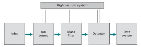
Fig. 9.1 Basic components of mass spectrometers.
