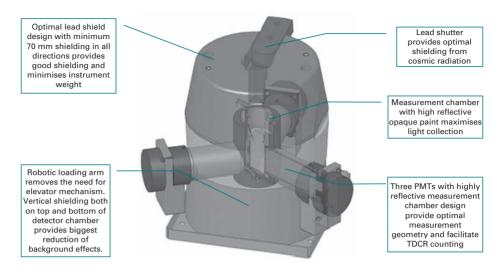
Fig. 14.8 The arrangement of photomultiplier tubes in a liquid scintillation counter. (Reproduced with permission from LabLogic; instrument shown is the Hidex 300SL.)
