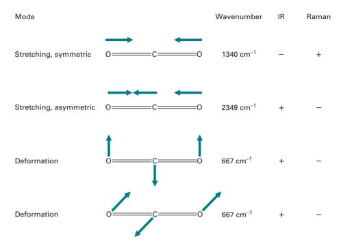
Fig. 13.2 Normal vibrational modes for CO<sub>2</sub>. For symmetric molecules that possess a centre of symmetry, bands that appear in the IR do not appear in the Raman spectrum.
