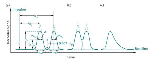
Fig. 11.1 (a) Chromatogram of two analytes showing complete resolution and the calculation of retention times; (b) chromatogram of two analytes showing incomplete resolution (fused peaks); (c) chromatogram of an analyte showing excessive tailing.
