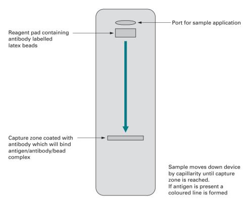
Fig. 7.16 Lateral flow device.
