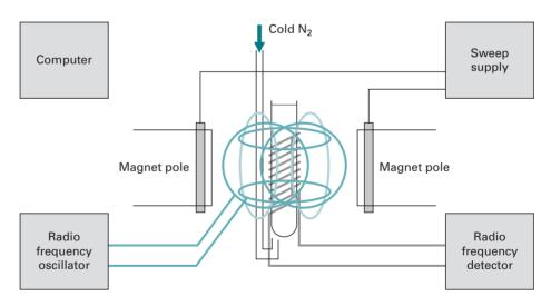
Fig. 13.11 Schematic diagram of an NMR spectrometer with cryoprobe.
