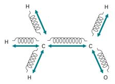
Fig. 13.1 Possible stretching vibrations in acetaldehyde.
