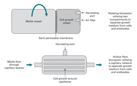
Fig. 7.8 Bioreactors for antibody production.
