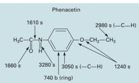
Fig. 13.3 FT–IR spectrum of phenacetin, the historically first synthetic fever reducer to go on the market. Bands at the appropriate wavenumbers (cm<sup>-1</sup>) are shown, indicating the bonds with which they are associated, and the type (s, stretching; b, bending).
