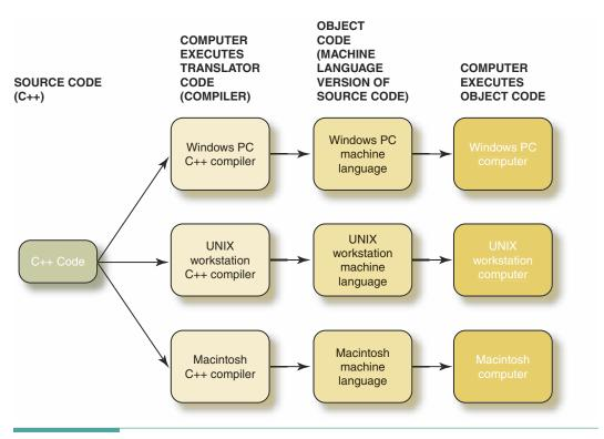
Figure 1.5 High-Level Programming Languages Allow Applications to Be Compiled on Different Systems
