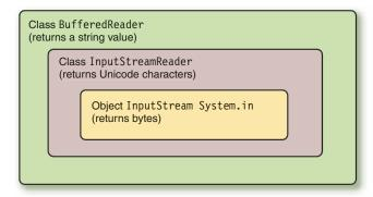
Figure 2.4 Layering of Classes for Java Input
