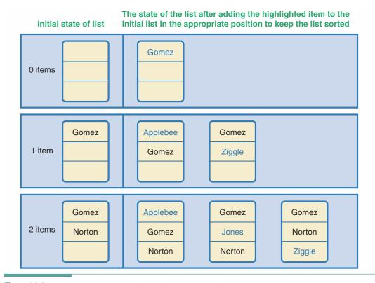
Figure 11.6 Inserting Items into a List So That Ordering Is Preserved
