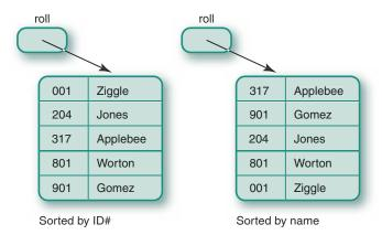
Figure 11.1 List Sorted by Two Different Keys
