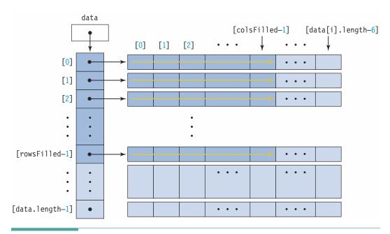
Figure 12.4 Subarray Processing by Row.
