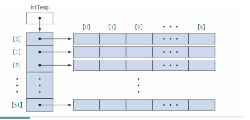
Figure 12.3 Java Implementation of hi Temp Array
