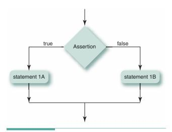
Figure 4.2 Selection (branching) Control Structure
