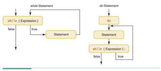
Figure 9.3 Flow of Control: while and do
