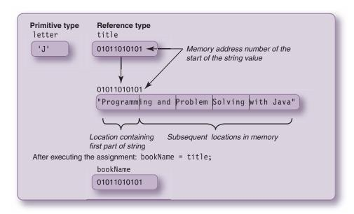
Figure 3.2 Primitive types and reference types
