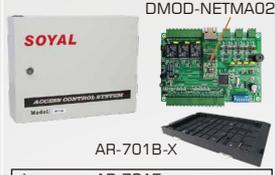
Two doors Wiegand controller / Wiegand to RS485 converter
