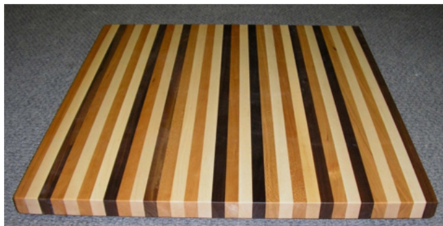
Butcher block top using three species: Maple, Cherry, and Walnut, finished clear.
