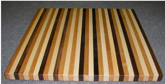
Butcher block top using three species: Maple, Cherry, and Walnut, finished clear.
