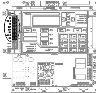
Figure 22: Relay wiring terminals
