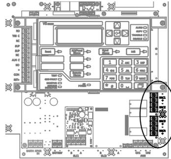
Figure 11: VS1 panel Class B NAC wiring
