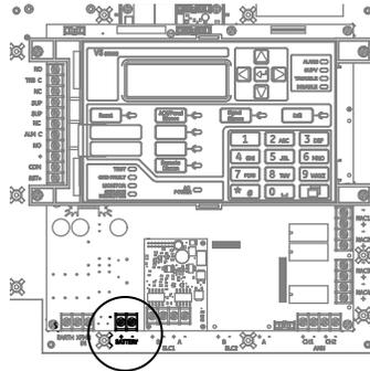
**Figure 9: Battery wiring**
