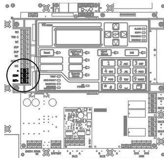
Figure 27: Auxiliary/smoke power output terminals
