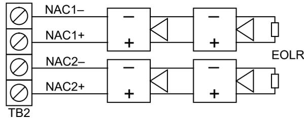
Figure 12: VS4 panel Class B NAC wiring
