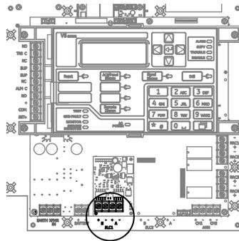
Figure 15: Class B wiring
