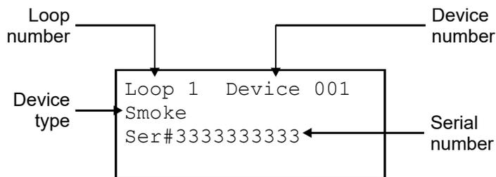
**Figure 51: Internal event (panel and loop events) details display screen**
