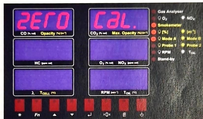
Figure 5. Zero calibration of the smoke head
