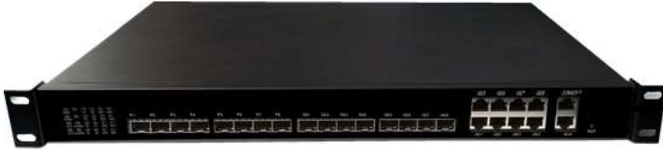
JD-AE28 provides 8GE(copper)and 8SFP slots Combo interface for uplink, and 8 EPON ports for downstream. It can support 512 ONU under 1:64 splitter ratio
